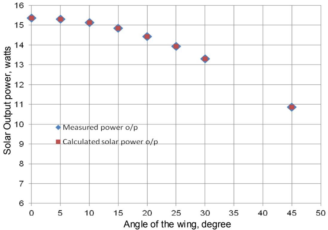
Fig.9 : Variation of Solar film O/P power with Incidence Change (Static Case): Comparison with calculated data from cosine relation
