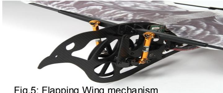
Fig.5: Flapping Wing mechanism
