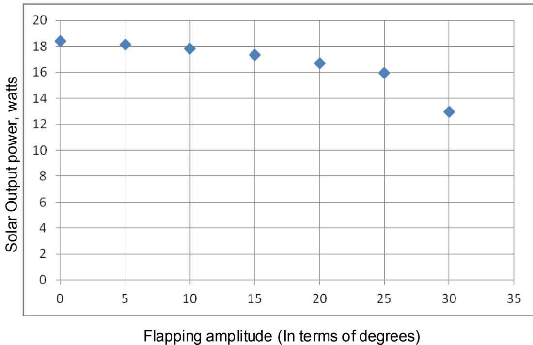
Fig.10 : Variation of Total Solar film O/P power with flapping
