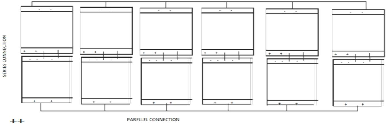
Fig.3: Solar film array configuration
