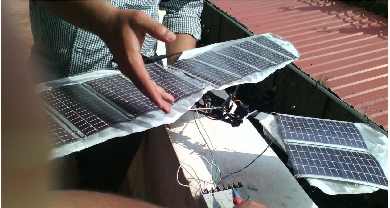
Fig.7: Fixing flexible solar films on flapping wing
