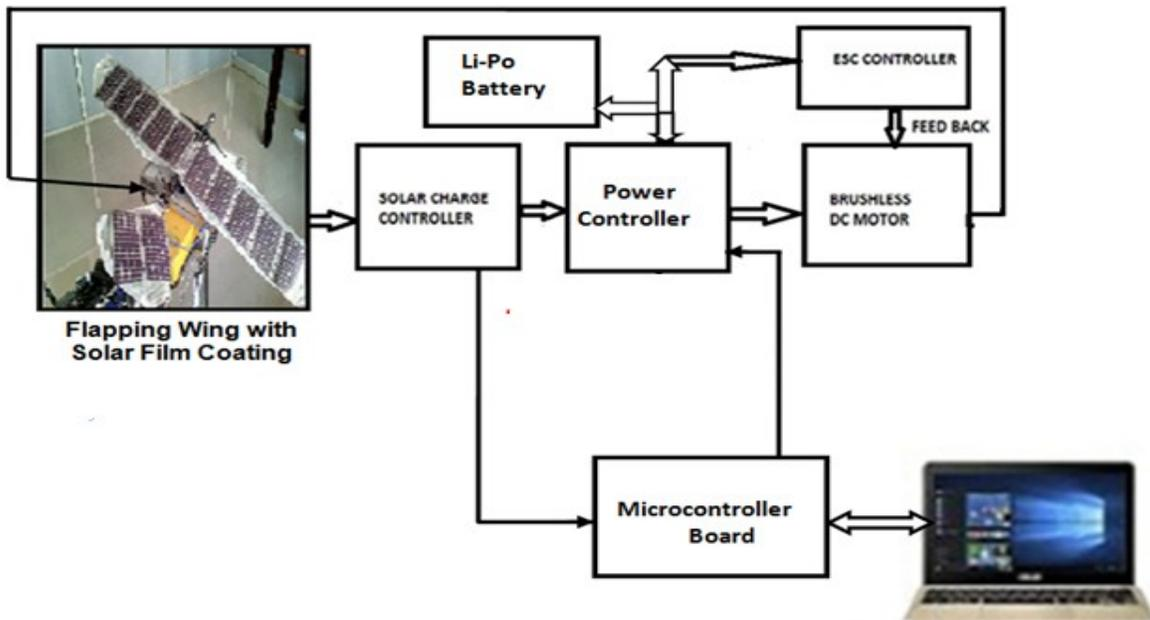
Fig.4 : Block schematic of power source with controller an data acquisition modules
