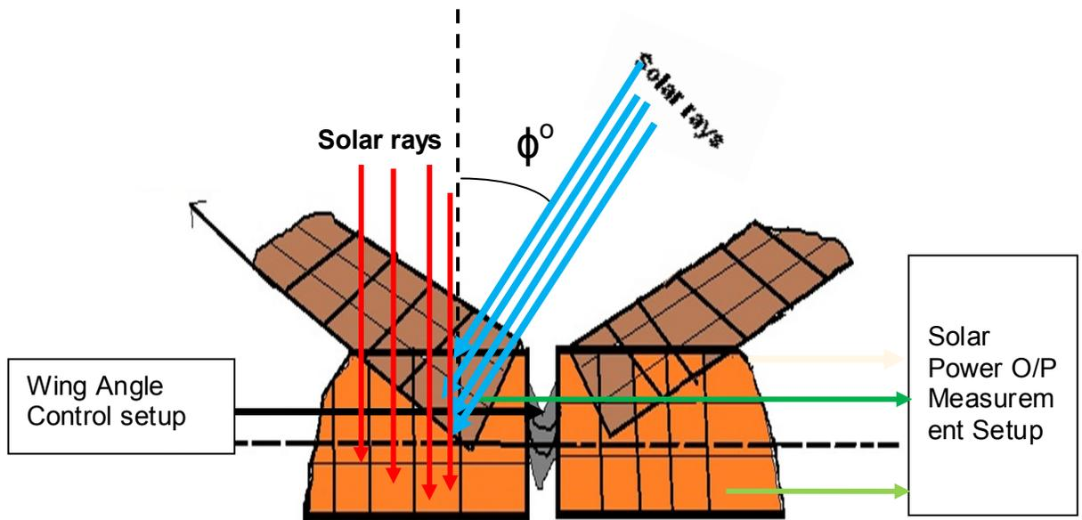
Fig.8: Setup for measurement of O/P power variation w.r.t wing angle changes
