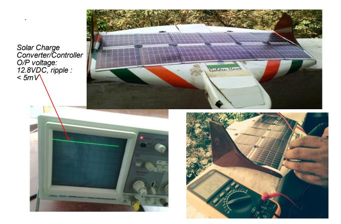
Fig.1 : Solar film test set up
