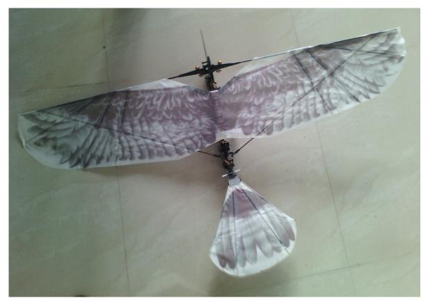
Fig.6: Flapping Wing Wing span: 1200mm, Chord :max 218mm, MAC :200mm, Tail:150X94mm2, Drive - Motor: BLDC
