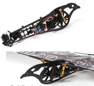
Fig.5: Flapping Wing mechanism
